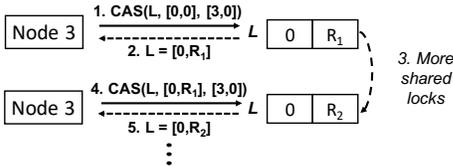
Figure 12: An example of a reader-writer starvation.
