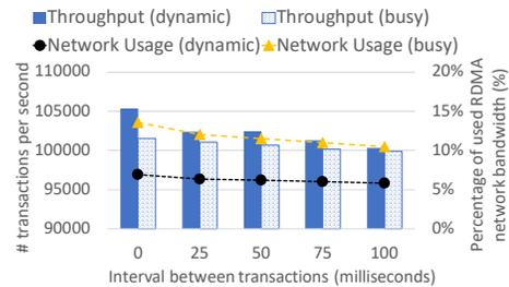
Figure 19: Transaction throughput and % of the RDMA network capacity used by DSLR with dynamic vs. busy polling.
